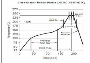
Soldering Profile for Lead Free Soldering 255-260°C
