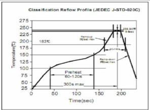
Soldering Profile for Lead Free Soldering 255-260°C
