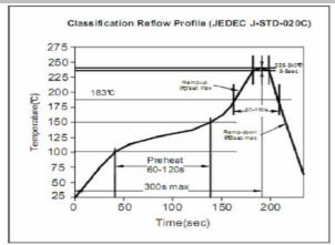
Soldering Profile for Lead Free Soldering 255-260°C
