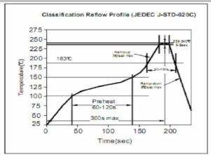
Soldering Profile for Lead Free Soldering 255-260°C
