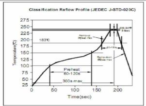
**Soldering Profile for Lead Free Soldering** 255-260°C
