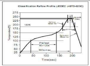
**Soldering Profile for Lead Free Soldering** 255-260°C
