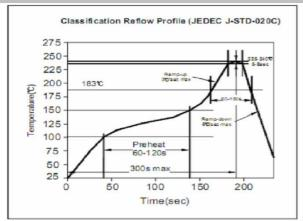
**Soldering Profile for Lead Free Soldering** 255-260°C
