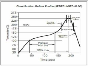
Soldering Profile for Lead Free Soldering 255-260°C
