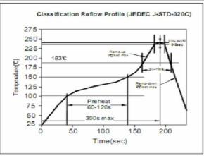
Soldering Profile for Lead Free Soldering 255-260°C
