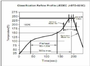
Soldering Profile for Lead Free Soldering 255-260°C
