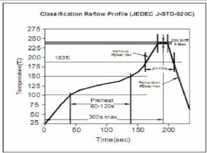
Soldering Profile for Lead Free Soldering 255-260°C
