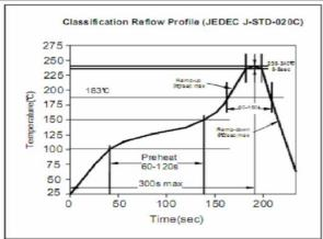
Soldering Profile for Lead Free Soldering 255-260°C
