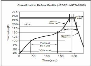
Soldering Profile for Lead Free Soldering 255-260°C
