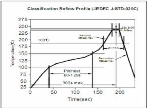
Soldering Profile for Lead Free Soldering 255-260°C
