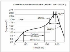
Soldering Profile for Lead Free Soldering 255-260°C
