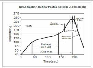
Soldering Profile for Lead Free Soldering 255-260°C
