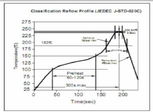
Soldering Profile for Lead Free Soldering 255-260°C
