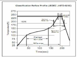
Soldering Profile for Lead Free Soldering 255-260°C
