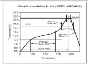
Soldering Profile for Lead Free Soldering 255-260°C
