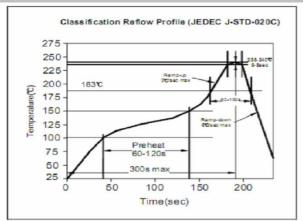
Soldering Profile for Lead Free Soldering 255-260°C
