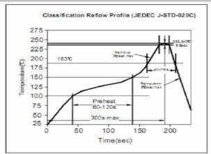
Soldering Profile for Lead Free Soldering 255-260°C
