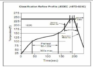
Soldering Profile for Lead Free Soldering 255-260°C
