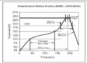
Soldering Profile for Lead Free Soldering 255-260°C
