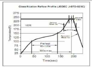
Soldering Profile for Lead Free Soldering 255-260°C
