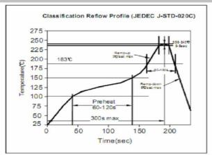
Soldering Profile for Lead Free Soldering 255-260°C
