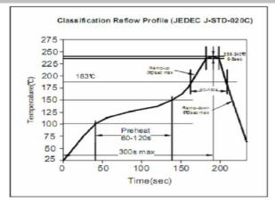
Soldering Profile for Lead Free Soldering 255-260°C
