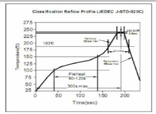
Soldering Profile for Lead Free Soldering 255-260°C
