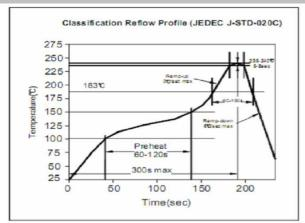
Soldering Profile for Lead Free Soldering 255-260°C
