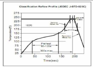
Soldering Profile for Lead Free Soldering 255-260°C
