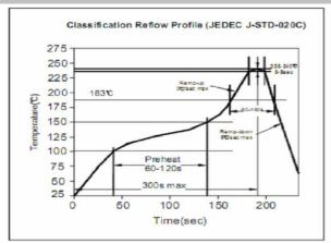
Soldering Profile for Lead Free Soldering 255-260°C
