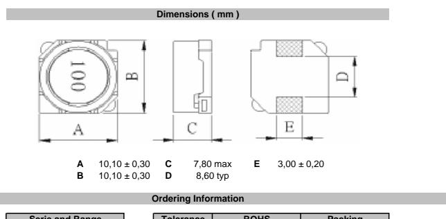
Serie and Range ROHS Packing Tolerance S49013-100 Μ R TR **K** = 10% R = ROHS BU = Bulk Ware **M** = 20% N = non ROHS TR = Tape Reel
