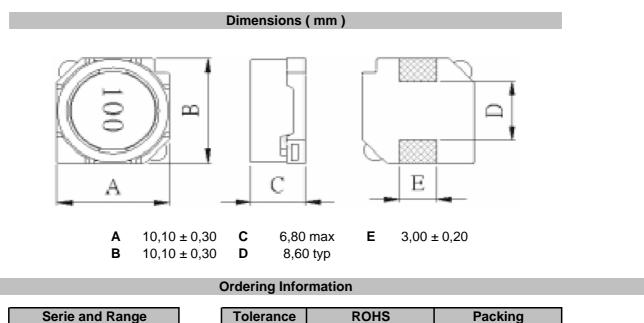
ROHS Packing Tolerance S49012-100 Μ R TR **K** = 10% R = ROHS BU = Bulk Ware **M** = 20% N = non ROHS TR = Tape Reel
