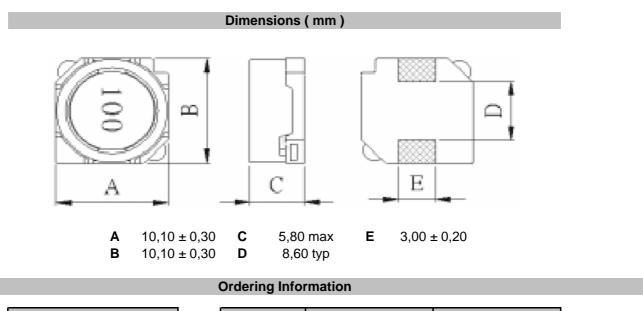
Serie and Range ROHS Packing Tolerance S49011-470 Μ R TR **K** = 10% R = ROHS BU = Bulk Ware **M** = 20% N = non ROHS TR = Tape Reel
