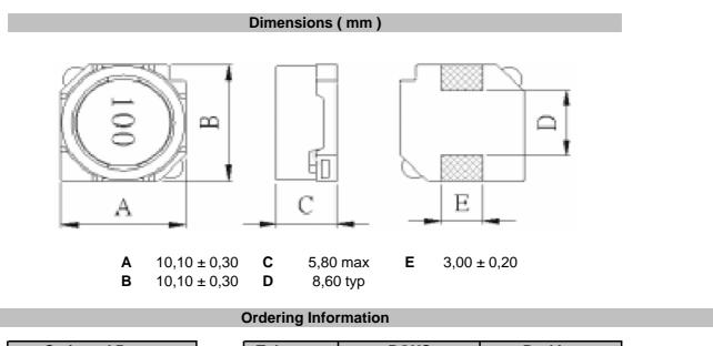
Serie and Range ROHS Packing Tolerance S49011-151 Μ R TR **K** = 10% R = ROHS BU = Bulk Ware **M** = 20% N = non ROHS TR = Tape Reel
