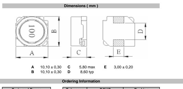
Serie and Range ROHS Packing Tolerance S49011-150 Μ R TR **K** = 10% R = ROHS BU = Bulk Ware **M** = 20% N = non ROHS TR = Tape Reel
