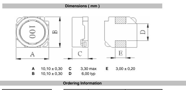
Serie and Range ROHS Packing Tolerance S49009-271 Μ R TR **K** = 10% R = ROHS BU = Bulk Ware **M** = 20% N = non ROHS TR = Tape Reel
