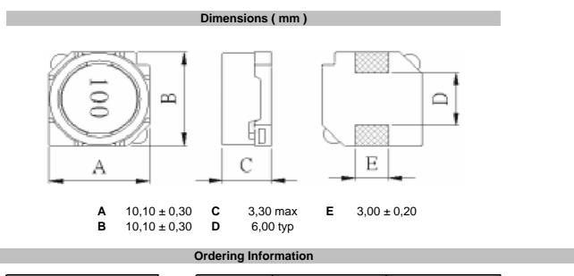
Serie and RangeToleranceROHSPackingS49009-221MRTRK = 10%R = ROHSBU = Bulk WareM = 20%N = non ROHSTR = Tape Reel
