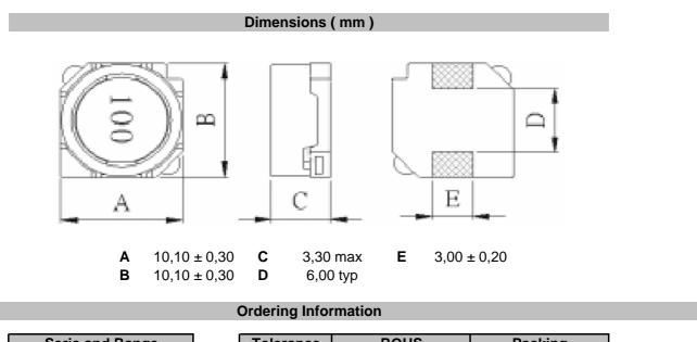
Serie and Range ROHS Packing Tolerance S49009-180 Μ R TR **K** = 10% R = ROHS BU = Bulk Ware **M** = 20% N = non ROHS TR = Tape Reel
