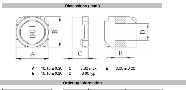
Serie and Range ROHS Packing Tolerance S49009-120 Μ R TR **K** = 10% R = ROHS BU = Bulk Ware **M** = 20% N = non ROHS TR = Tape Reel
