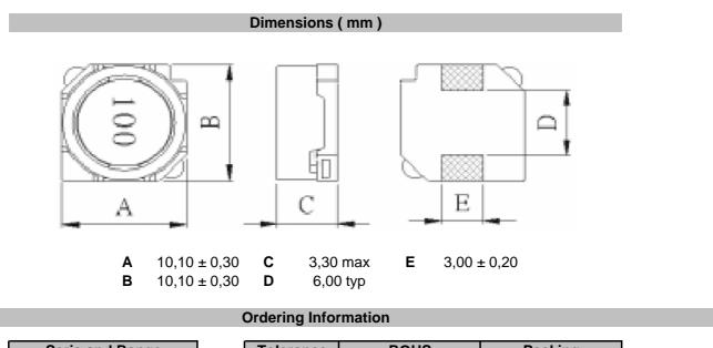
Serie and Range ROHS Packing Tolerance S49009-102 Μ R TR **K** = 10% R = ROHS BU = Bulk Ware **M** = 20% N = non ROHS TR = Tape Reel
