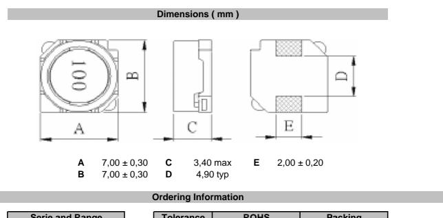
Serie and RangeToleranceROHSPackingS49008-3R3MRTRK = 10%R = ROHSBU = Bulk WareM = 20%N = non ROHSTR = Tape Reel
