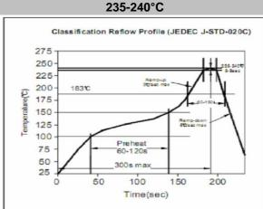
**Soldering Profile for Lead Free Soldering**
