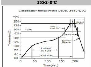
**Soldering Profile for Lead Free Soldering**
