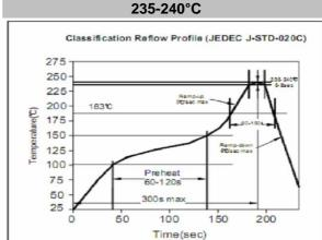
**Soldering Profile for Lead Free Soldering**
