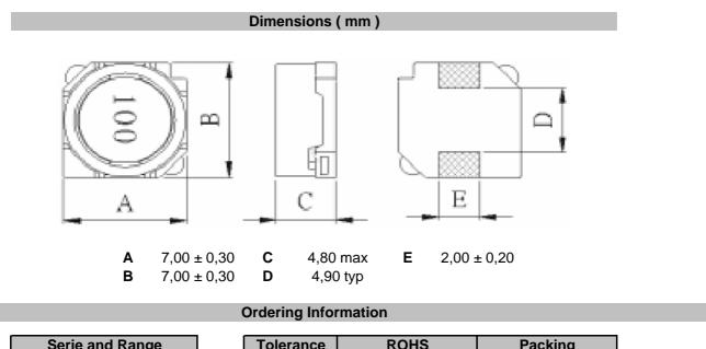
Serie and RangeToleranceROHSPackingS49008-101MRTRK = 10%R = ROHSBU = Bulk WareM = 20%N = non ROHSTR = Tape Reel
