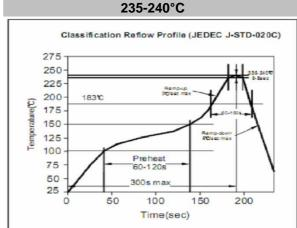
**Soldering Profile for Lead Free Soldering**
