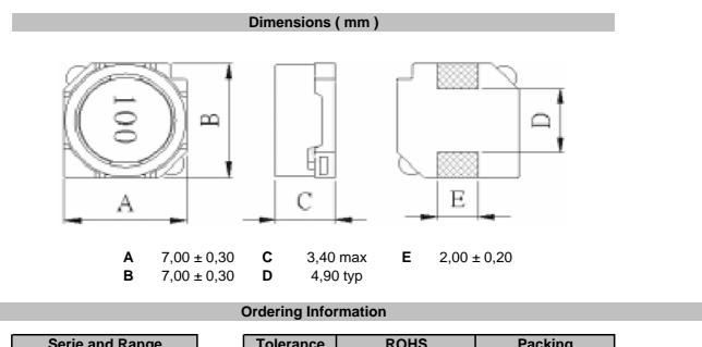
Serie and RangeToleranceROHSPackingS49007-6R8MRTRK = 10%R = ROHSBU = Bulk WareM = 20%N = non ROHSTR = Tape Reel
