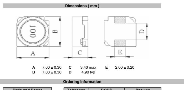
Serie and RangeToleranceROHSPackingS49007-680MRTRK = 10%R = ROHSBU = Bulk WareM = 20%N = non ROHSTR = Tape Reel
