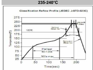
**Soldering Profile for Lead Free Soldering**
