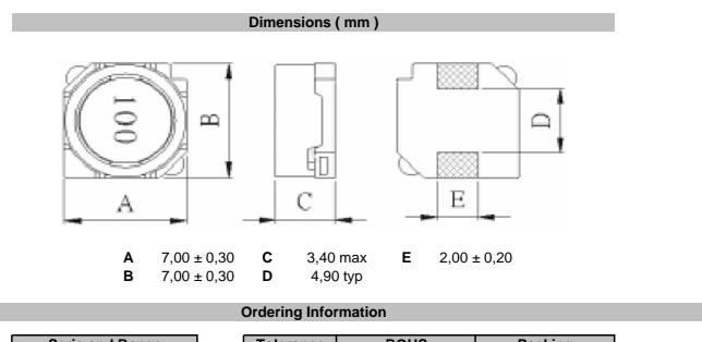
Serie and RangeToleranceROHSPackingS49007-102MRTRK = 10%R = ROHSBU = Bulk WareM = 20%N = non ROHSTR = Tape Reel
