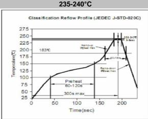
**Soldering Profile for Lead Free Soldering**
