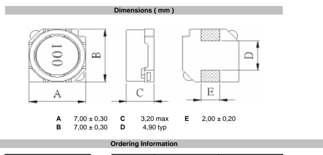
Serie and RangeToleranceROHSPackingS49006-220MRTRK = 10%R = ROHSBU = Bulk WareM = 20%N = non ROHSTR = Tape Reel
