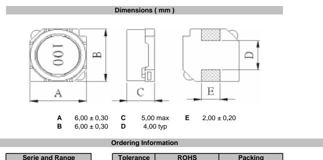
Serie and RangeToleranceROHSPackingS49004-561MRTRK = 10%R = ROHSBU = Bulk WareM = 20%N = non ROHSTR = Tape Reel
