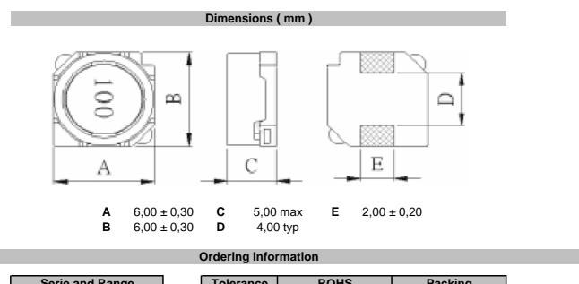
Serie and Range ROHS Packing Tolerance S49004-470 Μ R TR **K** = 10% R = ROHS BU = Bulk Ware **M** = 20% N = non ROHS TR = Tape Reel
